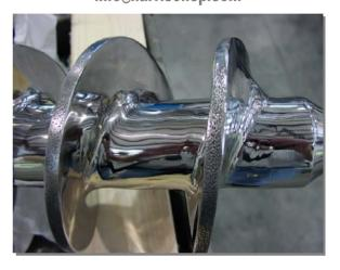
Solution: The required surfaces were polished to Harrison C-75 specifications. The shaft and flight faces of the conveyor screw were polished to reduce product adhesion. The OD surface was not polished so that the critical dimension was not altered. The customer saw a significant reduction of product buildup. Interval between cleaning shutdowns was increased. Time required to perform cleaning operation was decreased. Drive motors no longer experienced elevated loads.
