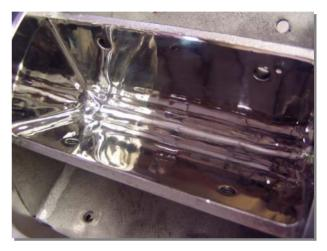
**Solution:** The required surfaces were polished to Harrison C-75 specifications. All internal surfaces of the rotor veins were polished to reduce product adhesion. The inlet and outlet of the rotor body were also polished. The customer saw a reduction of product buildup and a significant increase in product transfer rates.
